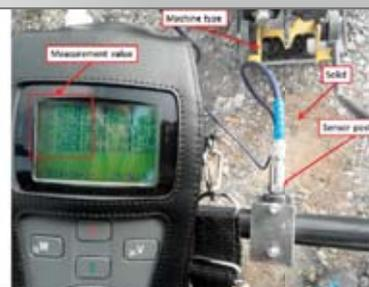
Equipment de test Larson Davis HVM 100 Tri-axial accelerometer.
